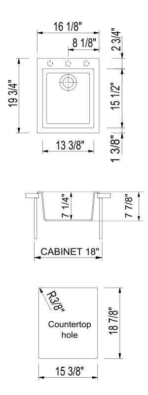
**NOTES:** Refer to installation instructions supplied with kitchen sink for undermount, or drop-in installations. Templates and installation kits provided with the sink.
