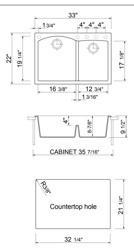
**NOTES:** Refer to installation instructions supplied with kitchen sink for undermount, or drop-in installations. Templates and installation kits provided with the sink.
