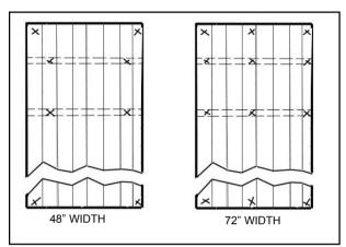
48 inch wide sheets should be all fastened to supports at all four corners and at points 6" in from the edges of each purlin support.
