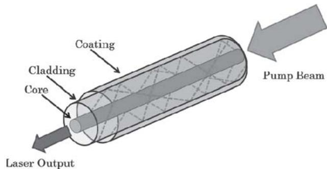
Fig. 1. Double clad fiber structure.
