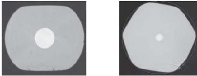
Fig. 8. Double-D and hexagonal shaped inner clad fiber fabricated at CGCRI.
