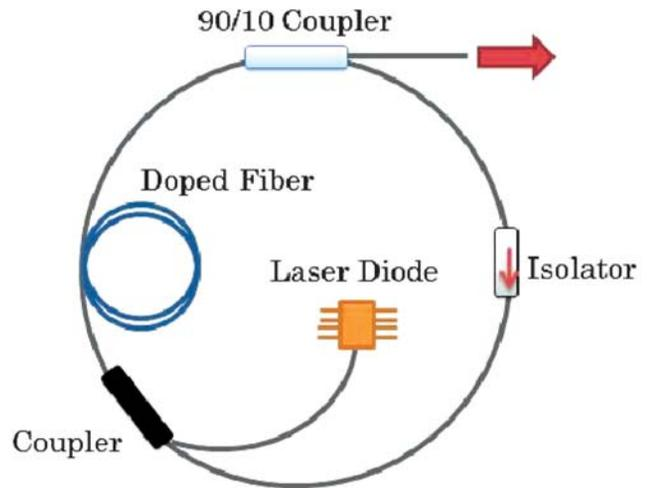
Fig. 4. Schematic of a ring cavity fiber laser.
