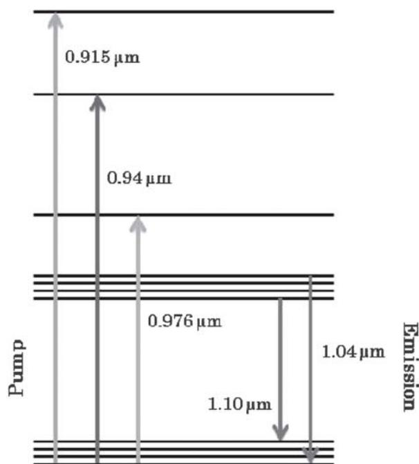
Fig. 6. Energy level diagrams of Yb in silicate glass.
