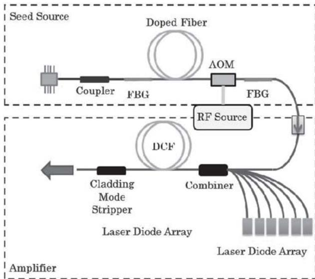
Fig. 5. Q-switched fiber laser seed source further amplified using a double clad fiber amplifier (MOPA configuration).
