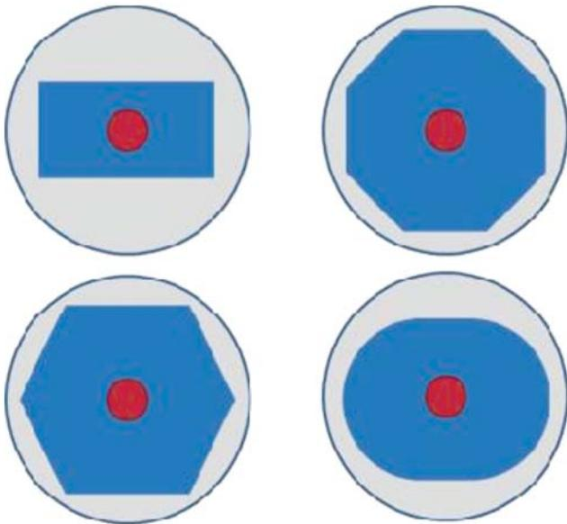
Fig. 2. Different inner cladding (blue region) geometry of double clad fiber.
