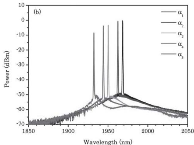
**Fig. 11.** Tunable laser spectrum in ring cavity from the Tm doped fiber laser designed at CGCRI.
