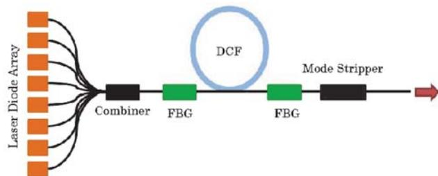
Fig. 3. Schematic of a diode pumped double clad fiber laser in linear or Fabry-Perot configuration.
