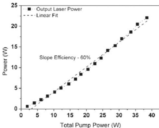
Fig. 9. Lasing characteristics of Yb doped fiber laser designed at CGCRI.
