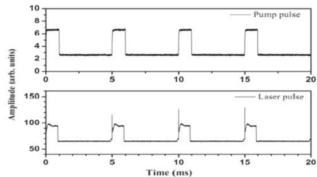
**Fig. 12.** Pump pulse and laser pulse for 20% duty cycle, 1 ms pulse width and 200 Hz repetition rate.
