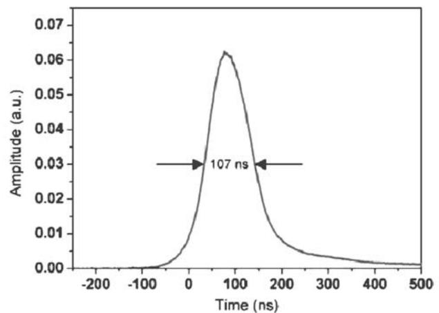
Fig. 10. Temporal shape of the output pulse from the Yb doped Q-switched fiber laser designed at CGCRI.
