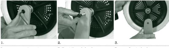
Loosen one capping nut.
