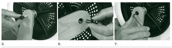
Insert threaded rod with capping nut on one end.
