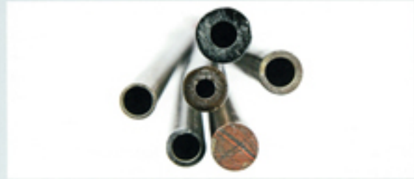
Vulcanite rod and tubes (usually 3' 6", 106mm in length), showing the internal and external diameters
