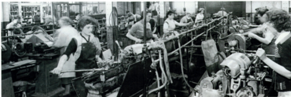
▲ The machine shop showing the capstans for drilling, threading and tapping the caps and barrels. "These girls were tough and were usually called Maggie!"
