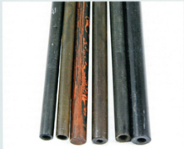
Vulcanite rod and tubes (usually 3' 6", 106mm in length), showing the internal and external diameters
