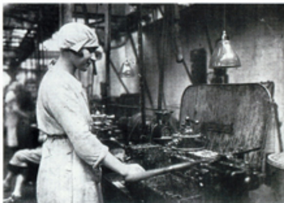
▲ Semi-automatic lathe used for boring, turning and finishing the vulcanite holders
