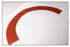
**4.** Note cutting height of selected dovetail on Dovetail Designer. Lay arcs on top of template, overlapping by at least height of selected dovetail.
