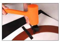
**9.** Alternatively, use Dovetail Punches to cut dovetails. See instructions for **DOVETAIL PUNCHES**
