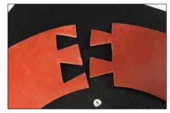
**8.** If arcs are significantly wider than single dovetail, consider multiple side-by-side dovetails per joint.
