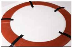
**5.** Position overlaps away from bolt-hole locations. As overlaps are made, tape down arcs to template on either side of overlap.
