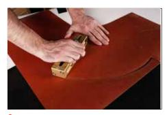
**3.** Cut multiple arcs of gasket material with desired OD and ID. Number of required arcs need to be greater than 360 degrees plus additional material for overlap.
