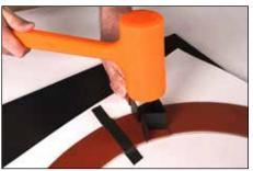
**6.** Position Dovetail Punch over each overlap. Tap with dead blow hammer to make initial indentation. Finish cut by striking Dovetail Punch with solid, flat blows. Top and bottom arcs will now have mating dovetails. Use utility knife to extend cut through if necessary. Tape dovetail joints together for easy handling.
