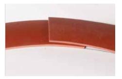
3. Select Dovetail Punch with cutting width slightly greater than difference between arc OD and ID. For example, for 1" (25 mm) wide arc, use Dovetail Punch No. 1 with cutting width of 1-1/4".
