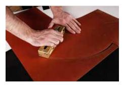
2. Cut multiple arcs of gasket material with desired OD and ID. Number of required arcs need to be greater than 360 degrees plus additional material for overlap.
