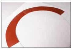
**4.** Note cutting height of selected Dovetail Punch. Lay arcs on top of template, overlapping by at least cutting height of selected Dovetail Punch.
