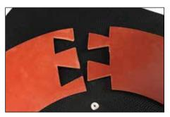
7. If arcs are significantly wider than single dovetail, consider multiple side-by-side dovetails per joint.
