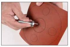
4. Insert offset pin through pilot hole.
