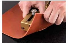
**8.** For thick or hard to cut gasket materials, make several shallow passes to complete through cut. Alternatively, cut halfway through gasket material, flip material over, and complete cut.
