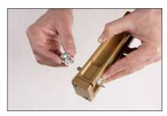
2. Slide pivot post indicator to desired outer diameter (OD) on scale 0" - 2" (51 mm) on bottom of cutter block. Tighten knurled nut.
