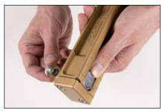
**9.** For small flange gaskets or washers, Slide pivot post indicator to desired inner diameter (ID). Tighten knurled nut. Repeat cutting steps.
