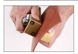
**7.** Hold cutting knob and material steady. With slight pressure, rotate cutter block clockwise relative to cutting knob to make cut.
