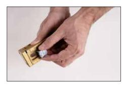
1. Insert pivot post with offset pin through cutter block, keeping offset pin towards cutting blade. Slide washer onto pivot post. Thread knurled nut loosely onto pivot post..
