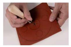
**3.** Insert center pin into center pin handle. Pierce center point of gasket material to create pilot hole.
