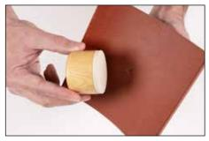
**5.** Flip gasket material over. Insert protruding offset pin into center hole on cutting knob.
