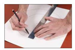
**6.** Place straight edge over pairs of opposite marks (for example 1 and 7). Using a pencil, extend straight line to PCD. Where straight line intersects with PCD is center point for bolt hole. Repeat for each pair of opposite marks.
