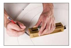
3. Pierce center point of paper or gasket material with center pin. Insert protruding center pin into recessed ferrule on cutting board. Using center point, use gasket cutter as compass by either holding a pencil against the outer edge, or with cutting blade to make very shallow cut. Scribe OD, ID and PCD.
