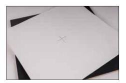
**1.** Lay blank sheet of paper or gasket material on cutting board. Locate approximate center point and mark.
