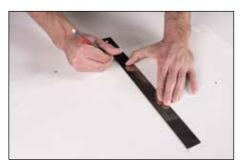
**2.** Measure and mark outer diameter (OD), inner diameter (ID), and pitch circle diameter (PCD) with straight edge.
