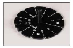
**4.** Position Bolt Hole Locator over center point. Insert center pin into recessed ferrule on cutting board. Press down firmly to hold Bolt Hole Locator in place.
