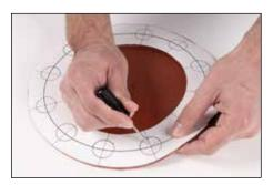
**9.** Lay template on top of partially finished gasket. Use piercing tool to transfer bolt hole center points onto gasket. Punch out bolt holes with hole punch.
