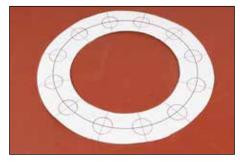
7. If gasket design is laid out on paper, using scissors cut out the paper template.
