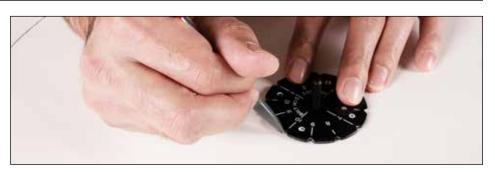
**5.** Note required number of bolt holes on desired gasket. Common configurations are 4, 6, 8, 12, and 24 bolt holes. Using a pencil, mark the following points on paper or gasket material utilizing notches around perimeter of Bolt Hole Locator:
