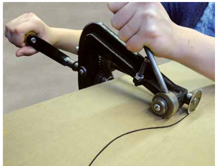
(Figure 9) To cut irregular shaped gaskets, mark the shape desired on the gasket material with a pencil or pen. Loosen the scale bar T-screw. Remove the scale bar, and manually feed the material through the cutters while operating the unit in the same manner as above. An additional set of hands may be needed to guide material.
