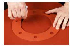
**1.** If existing gasket is available, using a pencil or marker, trace outline onto gasket material.
