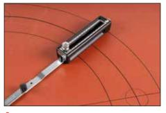
**6.** Position pivot post hole at tip of extension arm over center pin in gasket material. With the other hand, grip the cutter block, ensuring cutter block is lying flat on gasket material.
