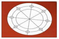
**3.** Another way to determine bolt hole locations is using a paper template with OD, ID and PCD. Transfer the bolt hole location center pins with piercing tool or pencil tip.
