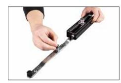
**5.** To cut gaskets over 25" (635 mm) diameter, add additional extension arm(s). Unscrew plastic threaded cap at end of previously installed extension arm. Position dual holes of next extension arm above threaded post and sleeved stud. Secure with plastic threaded cap.
