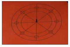
**5.** Choose center pin approximately ½" (12 mm) longer than thickness of gasket material. Push center pin through gasket material. Insert protruding center pin into recessed ferrule located in the center of cutting board. Lay gasket material flat on cutting board.
