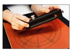
**8.** Position pivot post hole over center pin. Ensure cutter block is lying flat on gasket material.
