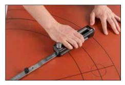
**7.** With slight downward pressure, rotate cutter block clockwise to make cut. Simultaneously press down on gasket material to prevent rotation.
