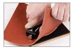
**10.** For thick or hard to cut gasket materials, make several shallow passes to complete through cut. Alternatively, cut halfway through gasket material, flip material over, and complete cut.
