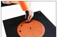
**11.** Punch out bolt holes using hole punch.
