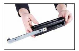
2. Completely unthread top thumb screw. Remove pivot post assembly. Remove bottom washer. Orient extension arm with hole labeled "pivot post hole" nearest cutting blade. Slide extension arm into groove on bottom of cutter block.
