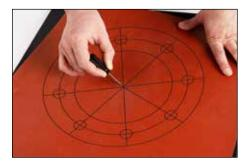
**4.** Create pilot hole by piercing center of gasket material with piercing tool.
