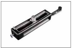
**4.** Gasket cutter can now cut up to 25" (635 mm) diameter. For example, cut 16" (406 mm) OD gasket by positioning pivot post indicator at 4" mark on cutter block scale (12" + 4" = 16").
