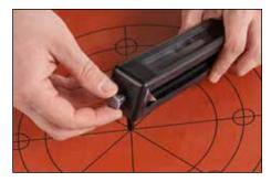
**6.** Loosen cutting blade thumb screw on cutter block. Position cutting blade to protrude slightly beyond thickness of gasket material. Tighten thumb screw.
