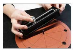
**12.** Loosen top thumb screw. Slide pivot post indicator to desired ID. Tighten top thumb screw.
