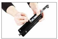
**3.** Insert pivot post through pivot post hole on extension arm and through cutter block. Slide washer onto pivot post. Thread knurled nut onto pivot post.
