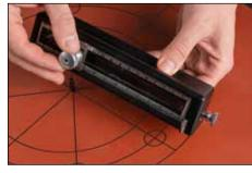
**7.** Loosen top thumb screw. Slide pivot post indicator to desired OD on cutter block scale. Tighten top thumb screw.
