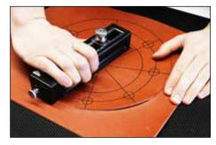
**9.** With slight downward pressure, rotate cutter block clockwise to make cut. Simultaneously press down on gasket material to prevent rotation.
