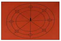
**5.** Insert protruding center pin into recessed ferrule located in the center of cutting board. Lay gasket material flat on cutting board.
