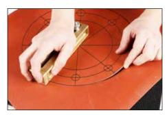
**10.** With slight downward pressure on cutting block, rotate cutter block clockwise to make cut. Simultaneously press down on gasket material to prevent rotation.
