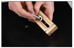
**3.** Insert thin-headed pivot post through single hole on extension bar and through cutter block. Slide washer onto pivot post. Thread knurled nut onto pivot post.
