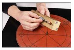
**13.** Loosen knurled nut. Slide pivot post indicator to desired ID. Tighten knurled nut. Repeat cutting steps.
