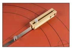
**6.** Position pivot hole at tip of extension bar over center pin in gasket material. Use the center pin handle to hold the center pin in place. With the other hand, grip the cutter block, ensuring cutter block is lying flat on gasket material.
