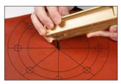
**9.** Position pivot post hole over center pin. Ensure cutter block is lying flat on gasket material.
