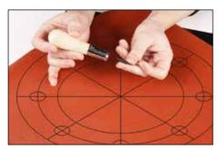
**4.** Choose center pin approximately ½" (12 mm) longer than thickness of gasket material. Insert center pin into center pin handle. Pierce center of gasket material. Disengage center pin handle.
