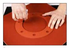
**1.** If existing gasket is available, using a pencil, trace outline onto gasket material.
