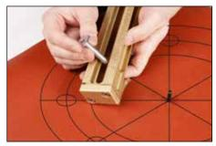
**6.** Insert thick-headed pivot post without offset pin through cutter block. Slide washer onto pivot post. Thread knurled nut loosely onto pivot post.
