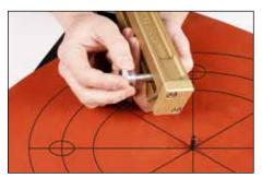
**7.** Slide pivot post indicator to desired OD on cutter block scale 0 - 13" (330 mm). Tighten knurled nut.
