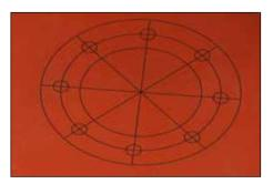
2. Otherwise, lay out outer diameter (OD), inner diameter (ID) and pitch circle diameter (PCD) directly onto gasket material. To determine bolt hole locations see LAYING OUT GASKETS WITH BOLT HOLES.
