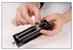
**8.** Loosen top thumb screw. Slide pivot post indcator to desired OD on cutter block scale. Tighten top thumb screw.
