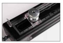
**3.** To cut a desired width, set indicator to double the width plus 3/16" (5 mm). For example, to cut 1" (25 mm) width, set indicator to 2-3/16" (55 mm).
