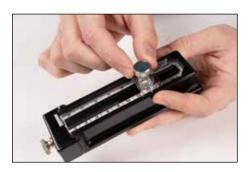
**13.** Loosen top thumb screw. Slide pivot post to desired ID. Tighten top thumb screw. Repeat cutting steps.
