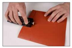
5. Place gasket material on cutting board. Align edge of gasket material with cutting board. Press down on gasket material. With slight downward pressure, run cutting block along edge of cutting board using flat side of pivot post block as a guide. For thicker gasket materials, use edge of gasket material itself as a guide.
