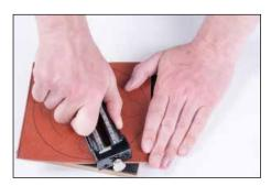
**10.** With slight downward pressure on cutting block, rotate cutter block clockwise to cut. Simultaneously press down on gasket material to prevent rotation.
