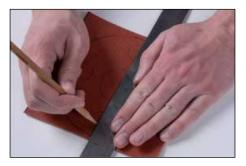
Otherwise, lay out outer diameter (OD), inner diameter (ID) and pitch circle diameter (PCD) directly onto gasket material. To determine bolt hole locations see LAYING OUT GASKETS WITH BOLT HOLES.
