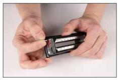
**4.** Choose center pin approximately ½" (12 mm) longer than thickness of gasket material. Insert center pin into silver hole at end of cutting block.
