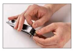
**7.** Loosen cutting blade thumb screw on cutter block. Position cutting blade to protrude slightly beyond thickness of gasket material. Tighten thumb screw.
