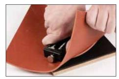
**11.** For thick or hard to cut materials, make several shallow passes to complete through cut. Alternatively, cut halfway through material, turn over, and complete cut.
