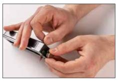
**4.** Loosen cutting blade thumb screw on cutter block. Position cutting blade to protrude slightly beyond thickness of gasket material. Tighten thumb screw.
