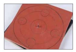
**6.** Insert protruding center pin into recessed ferrule located in the center of cutting board. Lay gasket material flat on cutting board.
