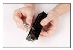
**1.** Completely unthread top thumb screw. Remove pivot post washer and indicator. Remove pivot post from cutter block.
