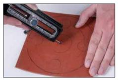
**5.** Using cutter block as a handle, pierce center of gasket material with center pin. Disengage cutter block leaving center pin protruding through gasket material.
