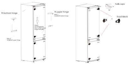
5) Remove the upper hinge of freezer door and plug pin.
