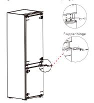
6) Remove the freezer door, the bottom hinge and the hole caps.
