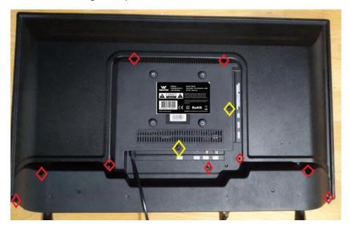
Step-2: Open the AV bracket's screw and take off the AV bracket. Then, take off the AC power cord from the connector, antenna connector, and all the other connectors.
