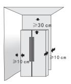
The refrigerator must be placed on hard, flat ground; if cushioning is needed, stable, hard, nonflammable cushion blocks shall be used.
