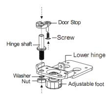
h) Install the adjusted lower hinge assembly to the left bottom side of the cabinet, and install the left front adjustable foot to the right bottom side of the cabinet.
