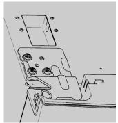
Remove the upper left hinge cover, connect the wire harness, and install it on the cabinet.
