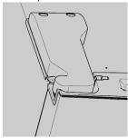
m) Remove the magnet from the door right side, and install it on the door left side
