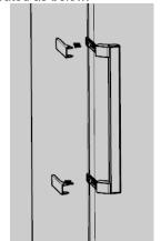
Install the handle on the other side of the door: rotate the handle by 180° degrees vertically, and install it on the opposite side of the door, as shown by the figure:
