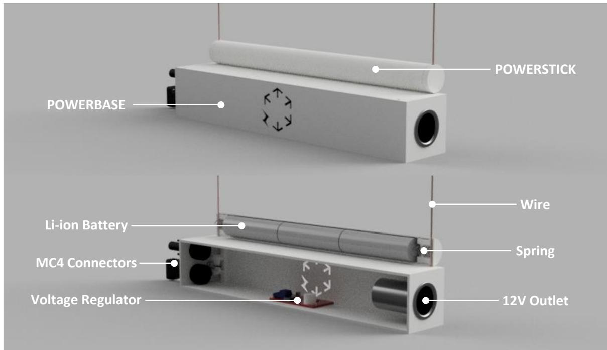
Figure 1: The POWERSTICK and POWERBASE
