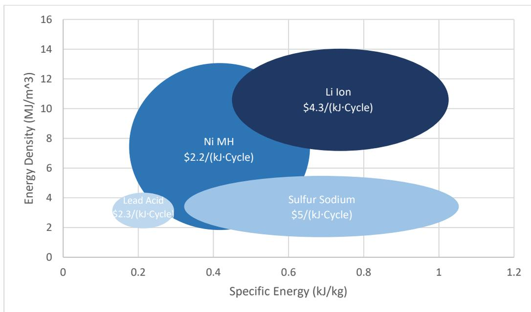
Figure 5 Specific Energy vs Energy Density for different battery chemistries (CES Edupack, 2016).
