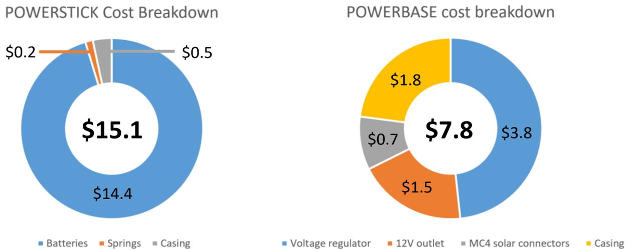
Figure 3: POWERCUBE Component Cost Breakdown (all prices in AU\$)
