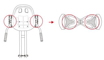
2. Secure your Hover-1 Buggy to your hoverboard using 2 of the included hook and loop straps. With the fastener side facing away from your hoverboard, thread the straps through the outside hole of each handlebar mount.
