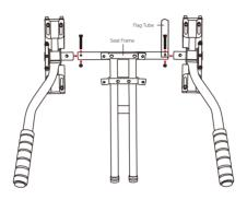
3. Insert the front frame into the seat frame. Adjust the front frame to your preferred length. Remove the black bolt and the first white washer from the end of each locker. Fully insert the screwed section of one locker into the seat frame holes. Add the white washer and black bolt back onto the locker once it is fully inserted and twist them on clockwise until they are tightly secured. Close the locker clamp tightly. Repeat these steps on the other side of the seat frame with the other locker.
