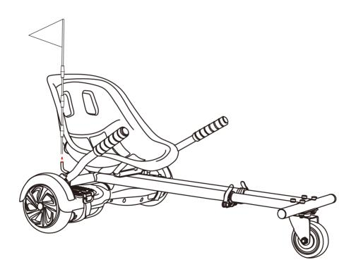
5. Your fully assembled Hover-1 Buggy should be attached to your hoverboard as shown below.
