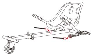
3. Wrap the straps underneath the hoverboard and pull them through to the other side. Insert the straps into the rear hole of the handlebar mounts. Fasten the front and rear sides of the straps. Make sure they are tightly secured to the hoverboard.
