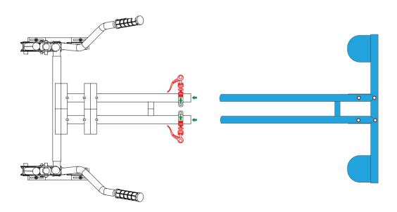
4. Align the holes of the seat with the holes of the seat frame as show below. Insert the M6 X16 screws. Attach the 20 mm washers and the 6 mm nuts to the bottom of each screw, under the seat frame. Twist the nuts on clockwise. Hold the 6 mm nuts still with the wrench while turning the screws clockwise with the larger hex key to tighten the screws. Make sure all 4 screws are tightly secured.
