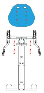
5. Align the holes of the wheel plate with the holes in the frame extension. Insert the M8 X 40 screws into each hole and attach the 6 mm lug nuts to each screw. Hold the 6 mm nuts still with the wrench while turning the screws clockwise with the larger hex key to tighten the screws. Make sure all 4 screws are tightly secured.
