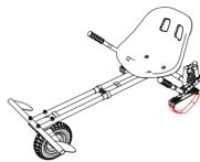
3. Wrap both straps under your hoverboard and pull them through to the other side. Insert the straps into the rear hole of the handlebar mounts. Fasten the front and rear sides of the straps. The rubber protectors on the straps should be centered underneath the hoverboard. Make sure they are tightly secured to the hoverboard.
