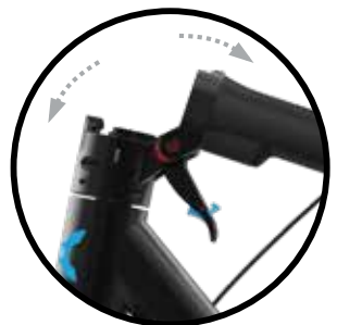
Release folding clip to fold steering column
