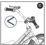
3. Use the multi-tool's hex key to loosen the screw inside the steering column and raise or lower the handlebars. Tighten the screw at the desired handlebar height. Tighten the other 2 screws at the top of the steering column with the hex key if needed.
