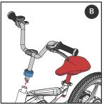
2. Place the rubber grommet (indicated in blue) on the steering column of the handlebar assembly as shown in Figure B. Insert the steering column into the front fork. Insert the seat pole into the frame and clamp the pole at the desired seat height.
