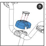
4. Line up the protective cover (indicated in blue) with the center of the handlebar assembly and attach it firmly. Push the centerpiece plate (indicated in gray) into the protective cover until it is locked firmly in place.
