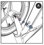
1. Loosen the outer lug nuts on each side of the front tire. Move the washers and outer lug nuts to the edge of the axle. Do not move the innermost lug nuts. Insert the front tire into the front fork. Insert the hooked washers into the front fork holes and move the rounded washers toward the wheel. Use a 15 mm wrench to tighten the outer lug nuts. Attach the black caps to the lug nuts.
