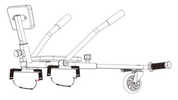
3. Wrap both elastic straps under your self-balancing scooter and attach the ends to the hooks on back of
