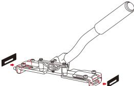
2. Using the two large screws and two large washers. Attach the handle bars to the appropriate sides of the seat frame as shown below. Tighten with included 6mm Allen wrench.
