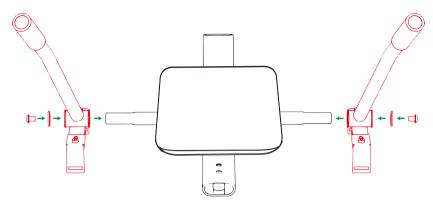
3. Insert the frame extension into the seat frame. Adjust to preferred length. Secure the frame extension in place using one twist knob.
