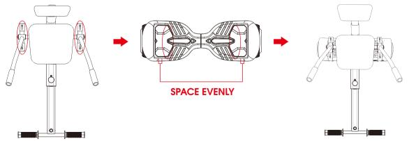
2. Using two elastic straps. Attach one end of each strap to the hooks on front of each pedal mount.
