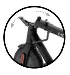
RELEASE FOLDING HINGE TO FOLD STEERING COLUMN
