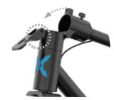
PULL RELEASE LEVER AWAY FROM THE STEERING COLUMN
