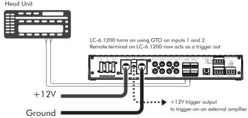
In this example, the head unit has a +12V trigger output that is connected to the LC-6.1200's remote input terminal. When the head unit is turned on, it will turn on the LC-6.1200 amplifier.
