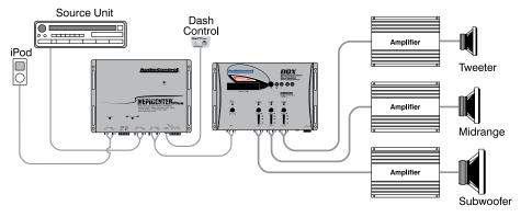
Figure 5: Two channel system with equalizer and crossover
