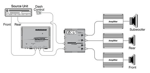
Figure 6: Four channel system with crossover
