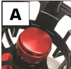
To remove the spool: on the frame loosen drag knob all of the way.
