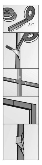
**Preparation of joint/application base:** The application area/pressure base should be as level as possible and cleaned (eg. Plaster leftovers removed completely). The joints should run parallel where possible (in some cases a re-plastering or re-profiling of the joints in older buildings could be necessary). The specified tape widths should not be exceeded or reduced and this also applies to use on uneven surfaces.
