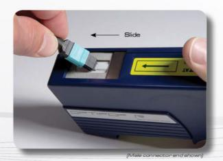
3. With cleaning cloth exposed, slide connector end face in the direction of the arrow.
