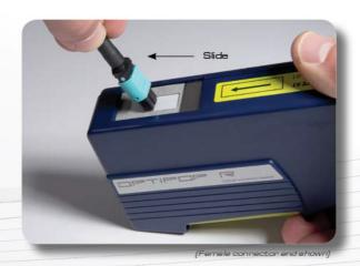
4. Keep connector perpendicular to cleaning surface.
