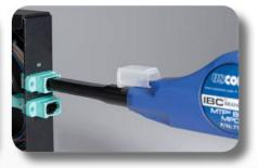
Push the cleaner forward inside the adapter until you hear a click, indicating the cleaning process is complete.
