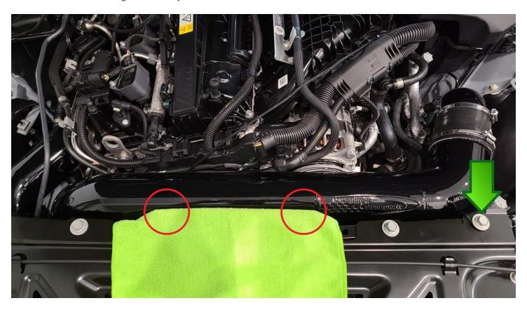
To start the front bumper removal process, peel up the weather stripping with the green arrows. Then remove the plastic clips circled in red.
