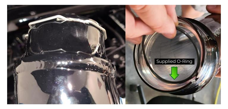
Now attach this short tube to the vehicle. Make sure the factory clip is secure and the tube is locked into place.
