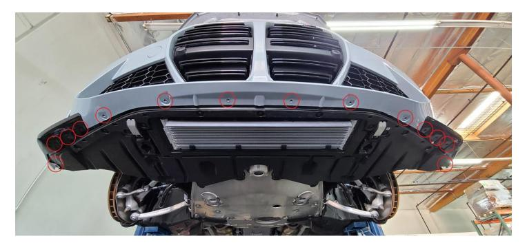
Now remove the four long black 8mm screws on the right and left side of the bumper cover that hold the bumper cover to the fender and have another person help you carefully pull the bumper cover off and move it to a safe location.
