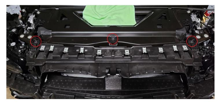
Now cut the upper plastic radiator shroud out by doing the lower cuts first with tin snips or similar tool. Then remove it from the vehicle by removing the plastic tabs and cut holes for the intake tubes to pass through on both sides.
