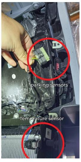
Now securely raise the front of the vehicle with jack stands or put in on a lift. Remove the right and left front wheels and remove the front half of the right and left plastic front wheel well covers by removing all the circled 8mm screws. Next disconnect the parking sensor and ambient temperature sensor in the wheel well. If your vehicle is equipped with active cruise control, there will be a 3<sup>rd</sup> sensor (not shown) to disconnect.
