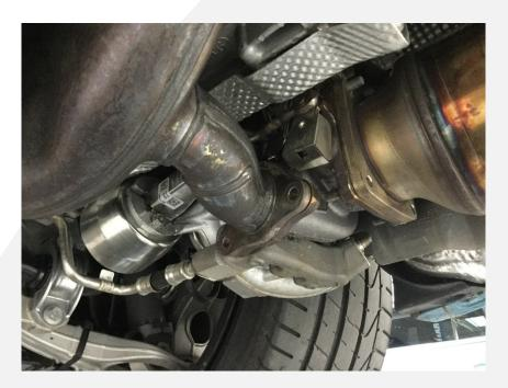
2. Remove the manifold mounting nuts using a 10mm triple square bit
