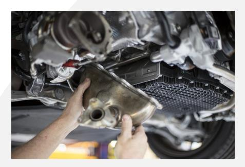
4. Installation is reverse of removal. Use supplied 13mm nuts, washers and bolts to replace the factory hardware as shown.
