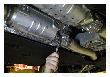
4. Using a 13mm socket, loosen and remove the bolts securing the mid-mounted hangar brackets (x2 on each side).
