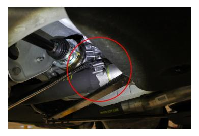
3. Using a 13mm socket, loosen and remove front flange nuts (x3 on each side).
