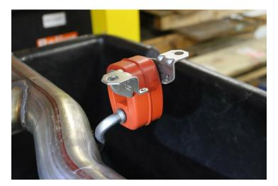
7. Slide rubber hanger onto Fabspeed X-Pipe.
