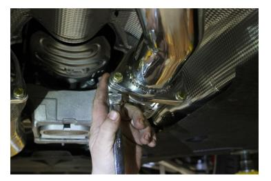
10. Tighten rear accu-seal clamps (x1 on each side) with a 15mm socket.
