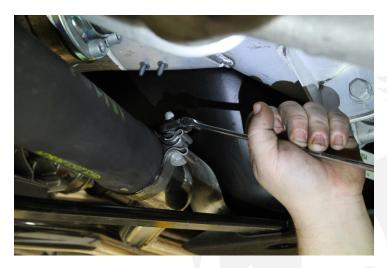
11. Re-insert and tighten hanger bolts (x2 on each side) with a 13mm socket.
