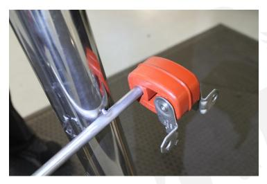
8. Position Fabspeed X-Pipe under vehicle and slide rear tubing into the muffler inlet tubes.
