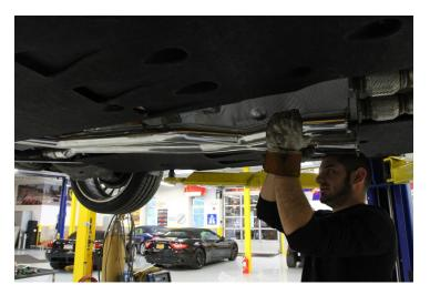
9. Insert and tighten front flange nuts (x3 on each side) with a 13mm socket.
