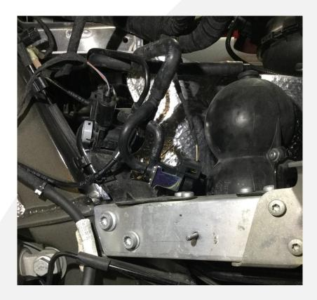
4. Locate the electrical connector from the factory solenoid.
