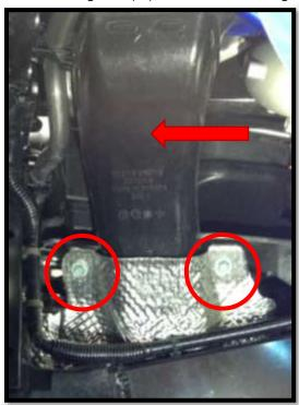
5. Remove heat shield. (x4) 10mm fasteners from back side. Lower two bolt holes are slotted. Bolts don't need to be fully removed.
