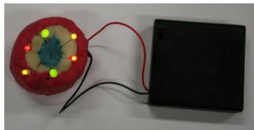
**Figure 1. A simple circuit created using a 6V battery pack, conductive and insulating dough, and LEDs.**
