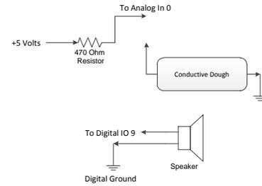
**Figure 4. Schematic for the Squishy Sound circuit.**
