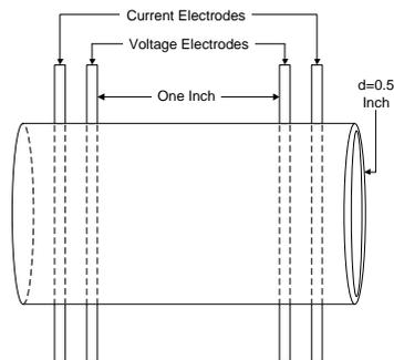
Figure 7. Test fixture used for resistivity testing of conductive dough.
