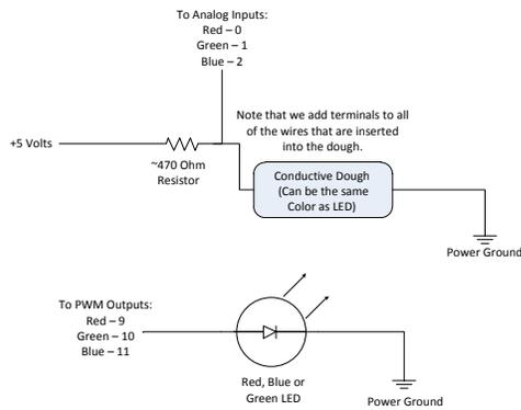
Figure 6. Schematic for the Squishy RGB Controller circuit.
