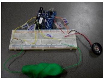
**Figure 3. A sound-producing circuit which uses conductive dough to control pitch.**
