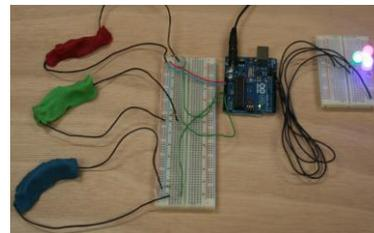
**Figure 5. A squishy interface for RGB LEDs.**
