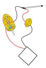
To flow power through the circuit and light up the LEDs, simply touch the magic wand to the magnets of the reed switch.
