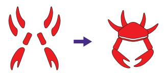
3 Attach the LEDs to the body of the crab. The longer wire from each LED should go into the bottom shell, and the shorter wire will insert into the top shell.
