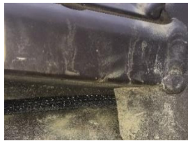
(Excel Boats) The best routing is through the gap in the back corner under the gunwale rail.
