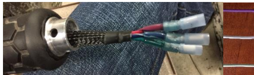
Red Blue to Purple Wire - Power Blue White to White Blue Wire- Up Green White to White Green Wire- Down
