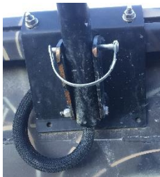
Routing Wires around the front of grab bar and across the back
