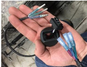
Connect Bullet Connectors
