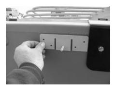
2- Bow: Depending on how much of the boat you want covered, you can attach the blind (a) at the front of the boat or (b) to the front of the bow platform. Many hunters leave the front bow section open for their dog and install at the (b) position. Modified V boats should use a crossbar which is sold separately. With the bolts pointing toward the inside of the boat, attach the front mount onto the center of the bow using the 5/16" self-tapping screws.
