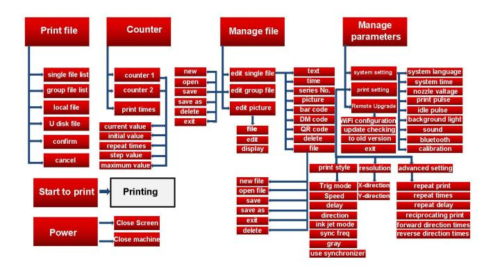
Note: this machine can operate on resistive touch screen directly, no need connect computer.
