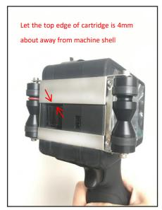
2. Push forward the cartridge slightly from back. Let the top edge of cartridge is 1mm about away from machine shell.
