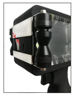
Let the top edge of cartridge is 4mm about away from machine shell
