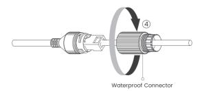
Step 4 Align the waterproof connector with the Ethernet port, then twist it clockwise to tighten the two parts.
