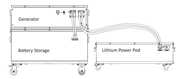
After you connect your Nature's Generator Powerhouse Lithium Power Pod to your Nature's Generator Powerhouse, you will experience an increased run time of approximately 200% by adding one Nature's Generator Powerhouse Lithium Power Pod, approximately 300% by adding two Nature's Generator Powerhouse Lithium Power Pods and 400% by adding three Nature's Generator Powerhouse Lithium Power Pods.
