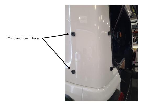
Step 6. Install mount with 1/4-20 x 7/8" bolts and Stainless flat washers. Tighten enough to fully expand well nuts.
