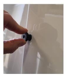
Step 4. Hold the propane mount up to the hard top on top of the first two rubber well nuts to mark the third and fourth holes.Insert bolts into the first two well nuts loosely then tip the mount out 3/16" to mark the third and fourth holes.
