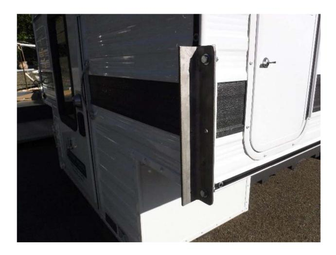
Be sure that the can holder is pushed next to the camper shell with no gap.
