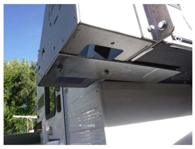
Some campers have nuts or bolts already coming through the area where the lower mounting plate might rest. You can cut some of the length off so that the existing bolts do not interfere with the lower mounting plate.
