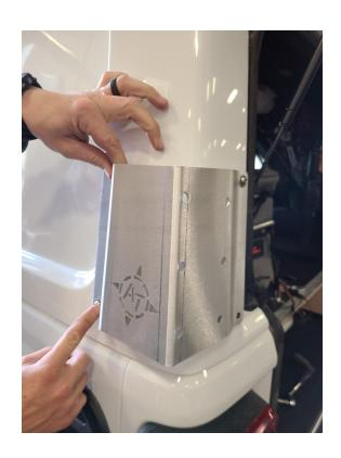
Step 5. Drill the third and fourth holes 1/4" and then 1/2" as before. Insert the two remaining well nuts.
