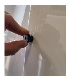
Step 4. Hold the propane mount up to the hard top on top of the first two rubber well nuts to mark the third and fourth holes.
