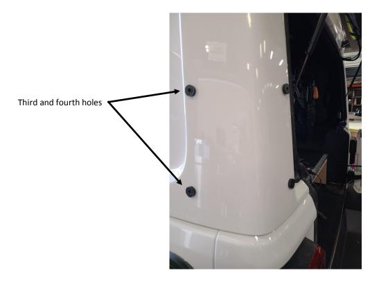
Step 6. Install mount with  $1/4-20 \times 7/8$ " bolts and Stainless flat washers. Tighten enough to fully expand well nuts.
