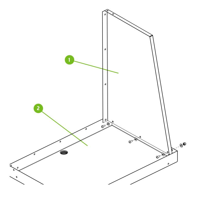
Slide the rear panel on the inside of the side panel flap and align the hole patterns to each other. You will need to place the spacer in between the rear panel and the rear of sink before attaching the hardware.
