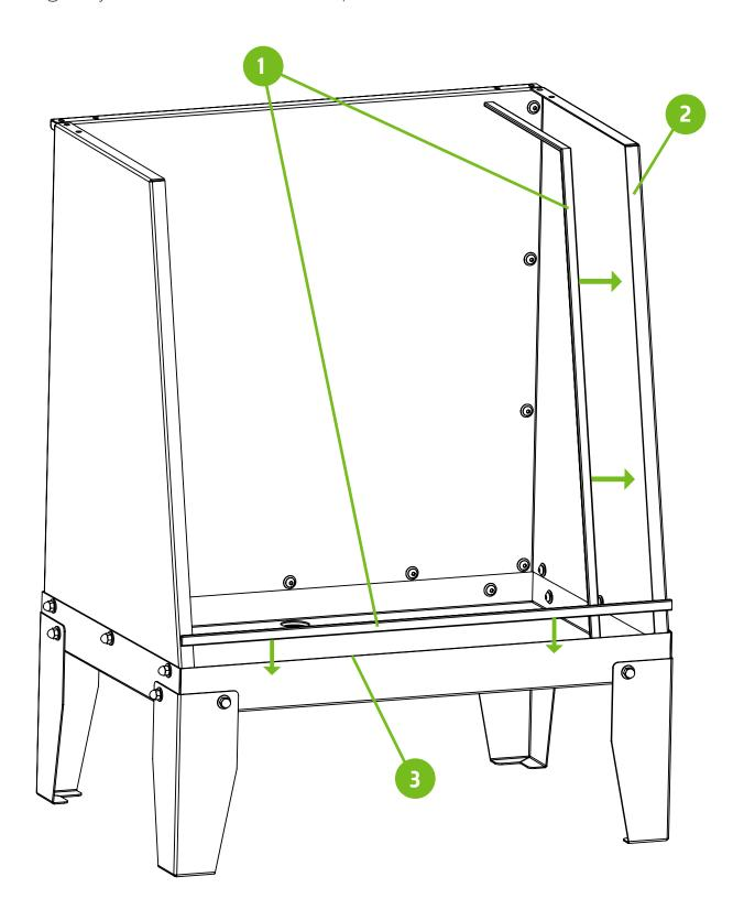
Install Gussets (1) to the side panels (2) and the rear panel (3). Fully tighten the hardware. No Neobond washers used in this step. Finally, use supplied caulk to seal all seams where water could leak. Allow to dry per caulking instructions.
