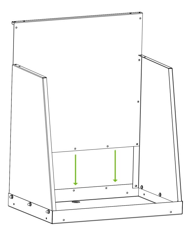
Install Rear panel (1) to the side panels (2) to the main sink body. Fully tighten the hardware. Neobond washers inside of the sink and standard flat washers outside of the sink.
