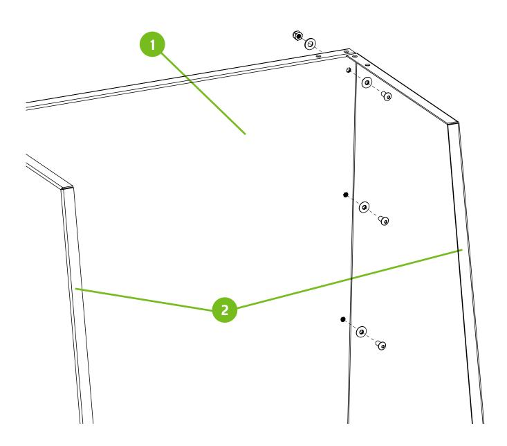
Install Legs **(1)** to the side panels to the main sink body **(2)**. Fully tighten the hardware. Neobond washers inside of the sink and standard flat washers outside of the sink.
