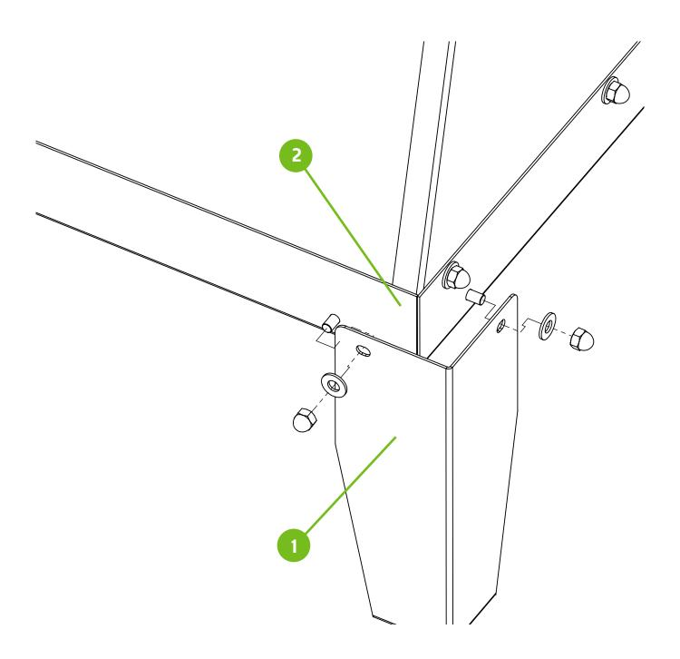
Install edge trim (1) to the side panels (2) and front lip of sink Body (3). Some trimming may be needed for this step.
