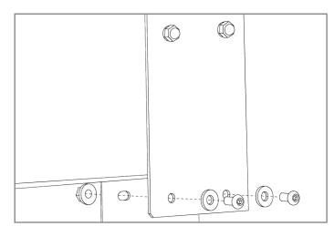
Install the legs uprights into the preinstalled leg clips. This will require the provided 1/4th inch bolts, washers and flanged nuts in the four holes-to-slots. Use the supplied 7/16th inch wrench and hex key to attach.
