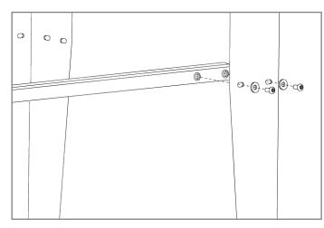
Install the aluminum tubular cross bars into the lower upright slots. This will require the provided 1/4th inch bolts and washers. Use the supplied hex key to attach.
